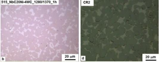
Guide rolls sintered at 1370 °C for 1 hour under vacuum (previous step at 1280 °C/1
