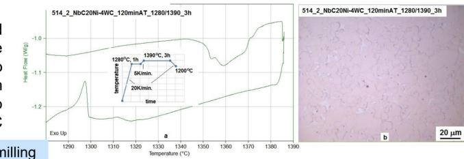
To anticipate the behaviour during typical industrial sintering cycles, thermal analysis (DSC and DIL) were carried out using two high temperature steps (1280°C/1390°C). The shrinkage profile was the same for samples (pressed at 200MPa) attritor milled for 15 or 120 minutes. As it was expected, the shrinkage for samples pressed at lower compaction pressure was higher.
