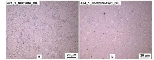
Optical micrographs (etched) for samples: (a) 421\_1, and (b) 424\_1
